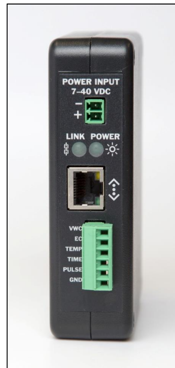
Fig 3. Prototype irrigation controller analog interface hardware.
