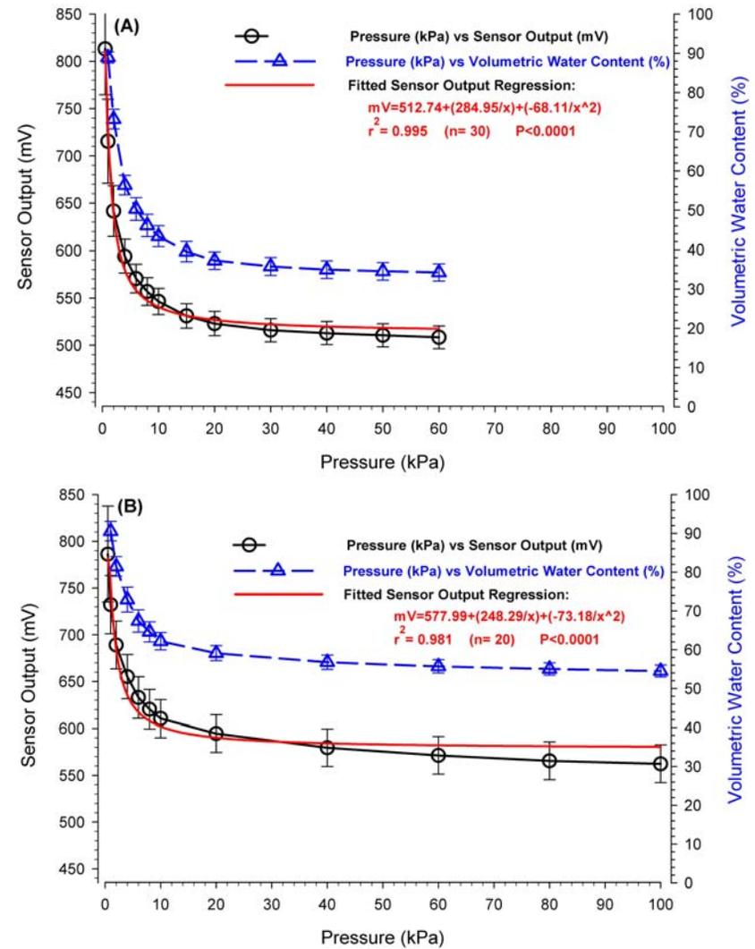
**Fig. 3.** Simultaneous sensor output (mV) and volumetric water content (%) vs. air pressure applied (kPa) for Ech<sub>2</sub>0-5cm sensors (Fig. 3A) and Ech<sub>2</sub>0-20cm sensors (Fig. 3B) in a 80:20 Peat : Perlite (Sunshine LC1) commercial substrate.
