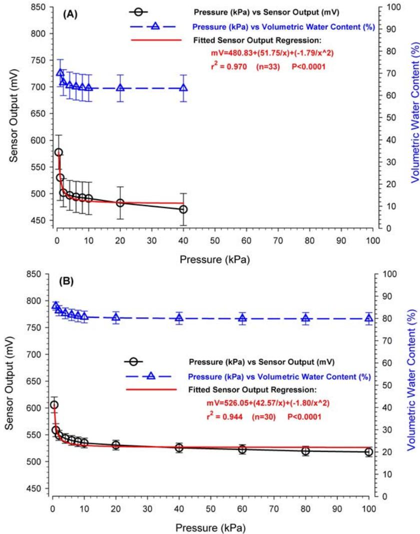
**Fig. 2.** Simultaneous sensor output (mV) and volumetric water content (%) vs. air pressure applied (kPa) for Ech<sub>2</sub>0-5cm sensors (Fig. 2A) and Ech<sub>2</sub>0-20cm sensors (Fig. 2B) in a 100% Perlite substrate.
