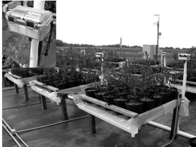
Fig. 1. Part of a twelve-node, 48 sensor network, showing an individual CMU wireless sensor node (inset, top left).
